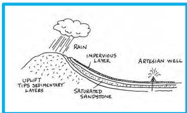
This well is artesian and water rises from 120 feet below the surface to a static level of 30 feet from the top. The cost of pumping water from a well is the cost of lifting the water from the static level to the surface, not from the entire depth of the well. The artesian nature of this well lifts the water naturally. A pump indicates minimal drawdown.
