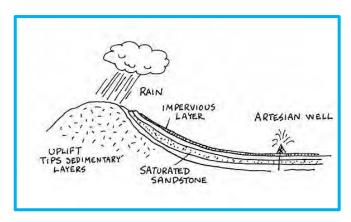
This well is artesian and water rises from 120 feet below the surface to a static level of 30 feet from the top.
