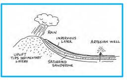
This well is artesian and water rises from 800 feet below the surface to a static level of 12 feet from the top. The cost of pumping water from a well is the cost of lifting the water from the static level to the surface, not from the
