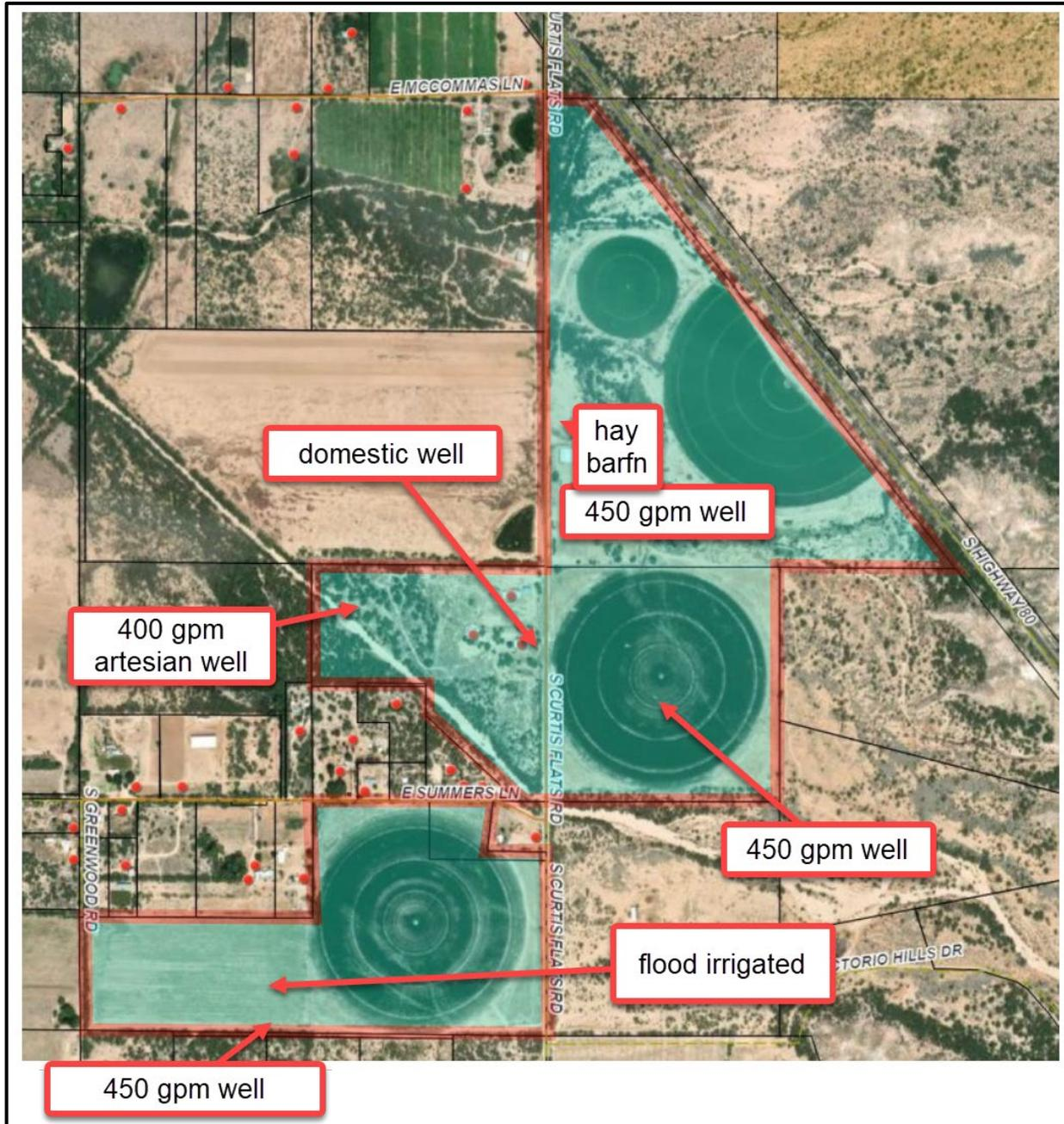
121-36-001A 400 GPM 800 foot deep **artesian**. This well is capped and has a hose bib and it produces > 20 gpm without a pump. Was designed for future lot splits and new homes.
